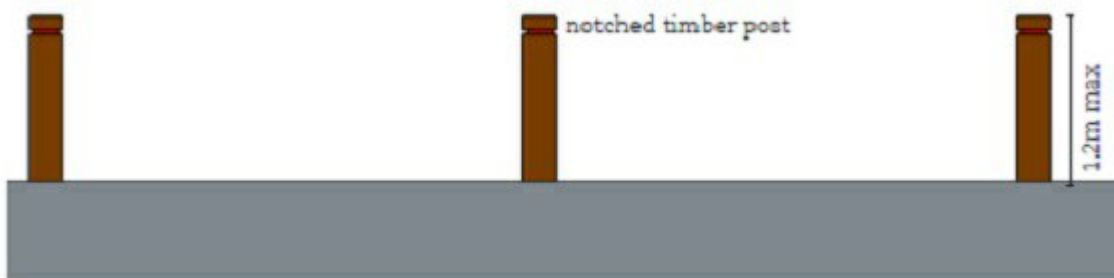
Figure 13 - Fencing Detail 3 - Public Open Space - Conservation
