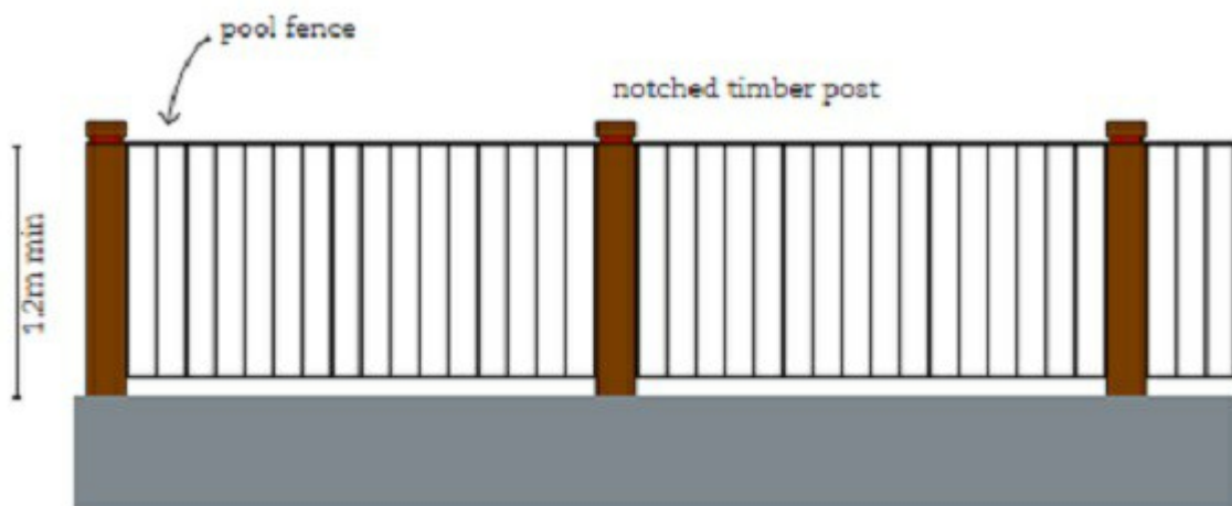
Figure 14 - Fencing Detail 4 - Green Infrastructure Zone
