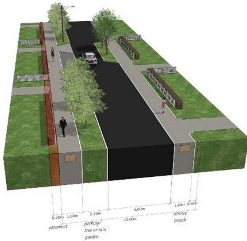
Figure 4 - Minor Residential Road
