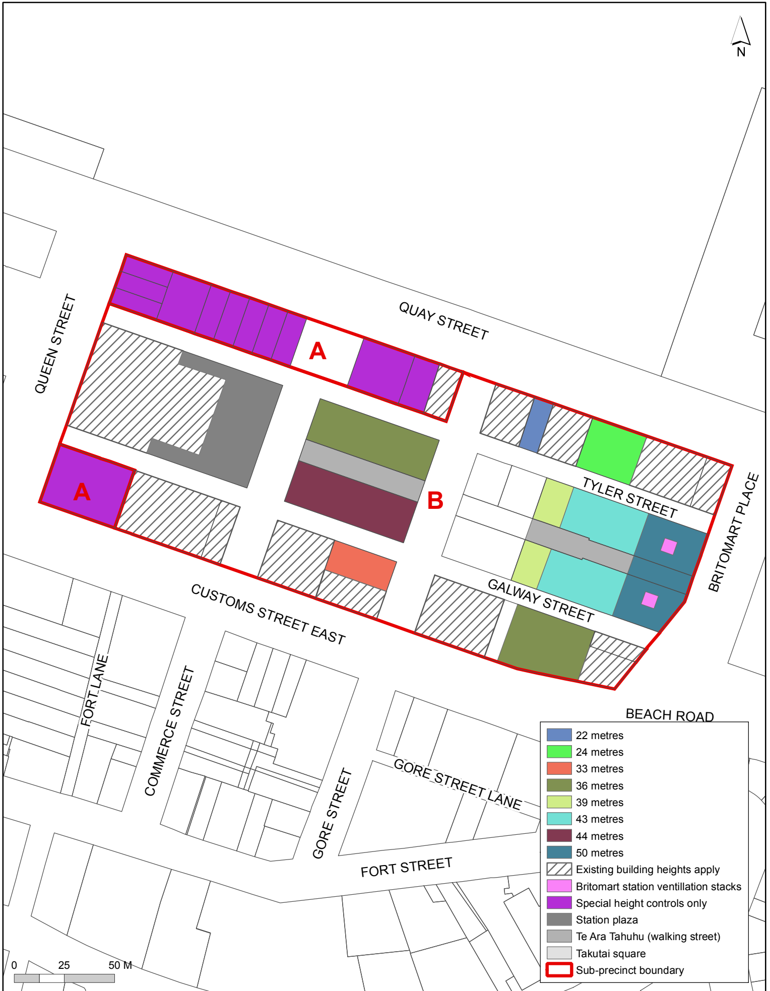
Britomart precinct plan 1: Building height controls
